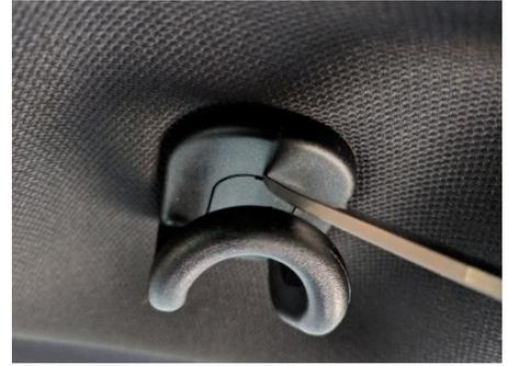
3. Pop open the screw cover on the driver side C pillar and remove the screw holding the cover. Remove the upper C pillar cover
