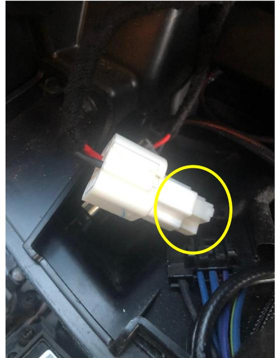
8. Plug the small two pin connector from the cigarette lighter t-harness into the two pin connector on the main cargo cam harness.
