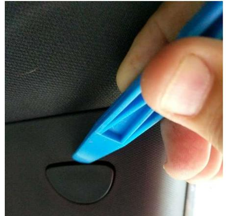
4. Remove the driver's side door thresholds on both the front and rear doors (where applicable). Rear threshold is shown in image to the right. Driver's side will have the kick panel attached to it.
