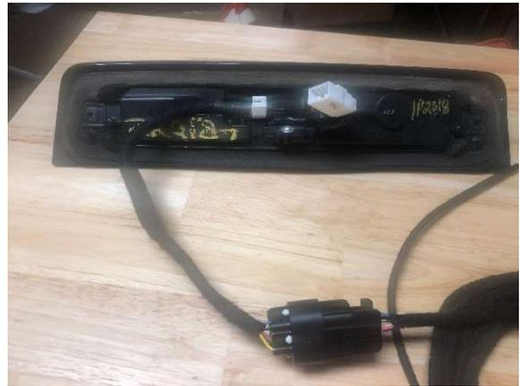
2. Connect the black connector from the harness to the black connector on the camera pigtail. It is fully inserted when a "click" is heard.
