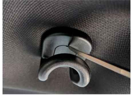
3. Pop open the screw cover on the driver side C pillar and remove the screw holding the cover. Remove the upper C pillar cover to reveal the i440 connector as shown below.
